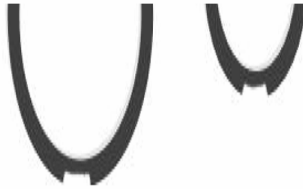
Figure 4.1 – Examples of bent D-shaped optical fibers [13].
