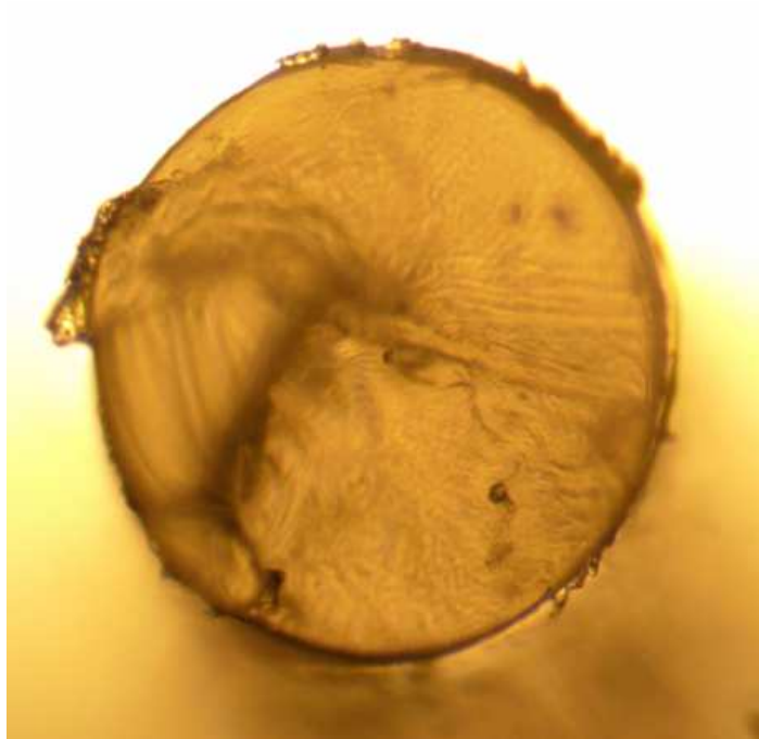
Figure 3.6 – An unpolished POF observed under microscope (transverse cross-sectional view).
